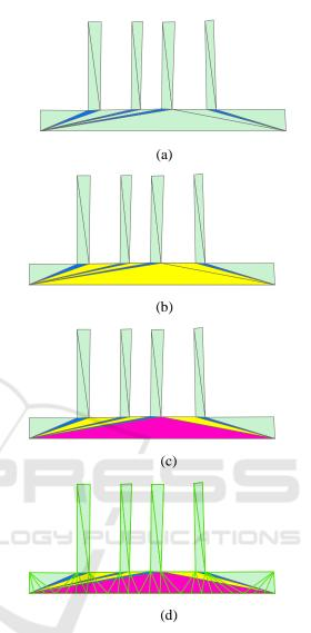
Figure 2: Long-edge adaptive densification. (a) Elongated Type III triangle, (b) Type II triangle with one edge as the boundary, (c) Local long edge to be densified, (d) Densify by densified step size.
