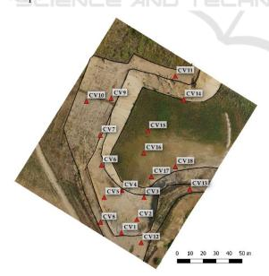
Figure 5: Configuration 1: all the GCPs used for BBA (red triangles).
