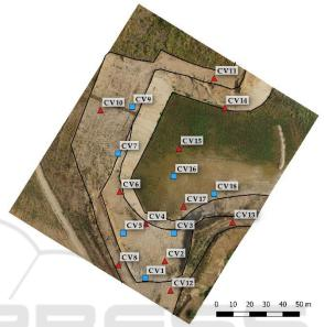
Figure 6: Configuration 2: 11 GCPs for BBA (red triangles) and 7 CPs for quality assessment (blue squares).
