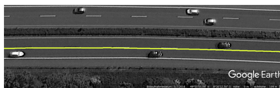
Figure 4: Reference line created from satellite images of the center dashed line.
