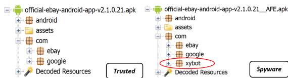
Figure 3: Android packages related to the trusted version of the official ebay application and the same application after the AFE injection (with highlighted the xybot malicious package).
