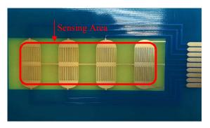
Figure 3: Fabricated sensor with gold coated surface finishing PCB.
