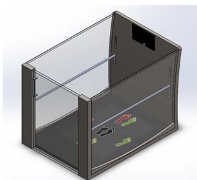
Figure 1: Representation of the water chamber of the ATP device.
