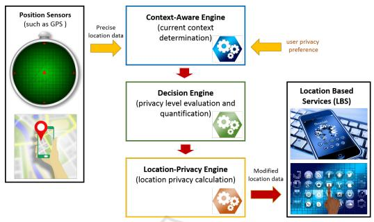
Figure 3: Proposed system architecture for Location-Privacy Assured IoT (LPA-IoT) Scheme.
