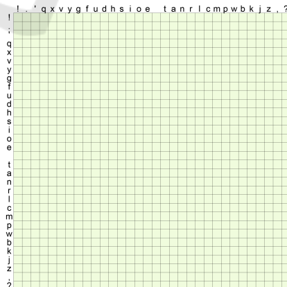
Figure 4: Central alignment of the examined keys. General frequency of the characters determine their position in the table. The more frequent ones appear in the middle, and when approaching the edges of the table, we encounter less and less frequent ones. Here, the space is considered as the most frequent one and glyphs as the least frequent ones.
