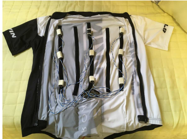
Figure 6: Front facing image of the prototype showing the internal part. In this image, the motors are configured as a 3x3 array.
