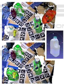
Figure 1: Multi-instance pose estimation example for a scene from the dataset of (Tejani et al., 2014). To the top is shown an example with non-optimized feature parameters, resulting in two correct (green) and one incorrect detection (red). The CAD model of the object is shown in the middle. Our parameter optimization improves the pose estimation algorithm, giving correct detection of all the three instances of the object shown at the bottom.
