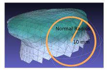
Figure 3: The important descriptor parameters for a single point in a point cloud. To the left is shown a representation of parameters: For each point, the Normal Radius is used to select nearby points for calculating the normal vector. All points within the Keypoint Radius is then used to compute the descriptor. In the middle the size of feature radius is shown, the 30 mm represent 10 % of the object size. To the right is shown a 10 mm normal radius, zoomed.
