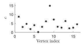
Figure 5: Correlation errors between the actual DP and the vertices of the map are shown. Here the vertex with the index 6 fulfills the required conditions and is chosen for the first position estimate.
