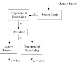
Figure 4: Wall Follower: Control method blocks representing the wall following algorithm.
