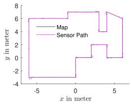
Figure 7: Example of a path along the boundary line generated using the presented wall following algorithm with  $a_{\mu} = 0.7$ ,  $a_{\nu} = 0.7$ , M = 100 and a sensor noise of 10%.
