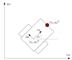
Figure 3: A differential drive robot within the 2-dimensional world frame given by  $\mathcal{W}$ . The robots main frame  $\mathcal{B}$  is determined by the frame for the odometry. The robots position is given by  $x_r$ ,  $y_r$  and the sensor position by  $x_s$ ,  $y_s$ .
