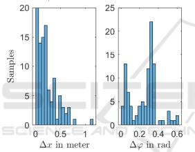
Figure 13: Evaluation results for map 2: Histogram of the difference between position and orientation estimate and true position and orientation after matching through shape comparison with  $\mu_{\Delta x} = 0.23$ ,  $\mu_{\Delta \phi} = 0.25$ ,  $\sigma_{\Delta x} = 0.20$ ,  $\sigma_{\Delta \phi} = 0.15$ .
