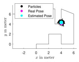
Figure 6: Sampled Particles: Particles have been sampled around the first pose estimate generated using land navigation.
