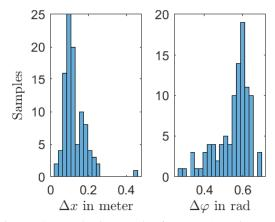
Figure 12: Evaluation results for map 1: Histogram of the difference between position and orientation estimate and true position and orientation after matching through shape comparison with  $\mu_{\Delta x} = 0.13$ ,  $\mu_{\Delta \phi} = 0.55$ ,  $\sigma_{\Delta x} = 0.06$ ,  $\sigma_{\Delta \phi} = 0.09$ .
