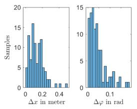
Figure 14: Histogram of the difference between position and orientation estimate and true position and orientation after the systematic search using the particle filter with  $\mu_{\Delta x} = 0.13$ ,  $\mu_{\Delta \phi} = 0.04$ ,  $\sigma_{\Delta x} = 0.086$ ,  $\sigma_{\Delta \phi} = 0.04$ .
