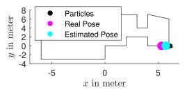
Figure 15: Randomly sampled particles around the position estimate  $x_{est}$ .
