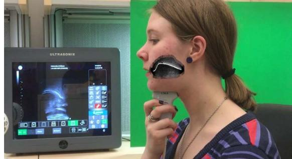
Figure 4: An instructor is pronouncing a list of words and her face and voice are recorded by the camera as well as ultrasound video. Manually, cropped ultrasound video and the tongue contour extracted (green line) from that video are superimposed with the video from the camera.
