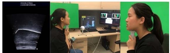
Figure 5: A learner is pronouncing a list of words after hearing the voice and watching the video from the instructor. The white color line is extracted from ultrasound data automatically.
