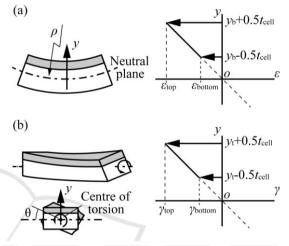
Figure 3: Schematic image of strain distribution in a cell. (a) Strain distribution during bending stimulus. (b) Shear strain distribution during torsion stimulus.
