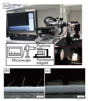
Figure 6: Images of experiment. (a) Experimental setup to measure inclination angles of microstructures. (b) Inclination of the microstructure for bending stimulus under  $H_{\text{ext}} = 343$  kA/m. (c) Inclination of the microstructure for torsion stimulus under  $H_{\text{ext}} = 343$  kA/m. Scar bars, (b) and (c): 100 µm.
