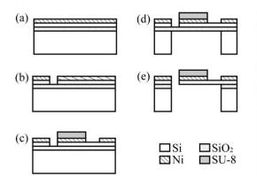
Figure 4: Cross-sectional diagrams of the fabrication process. (a) Sputtering Ni layer. (b) Etching Ni and device-Si layer. (c) Etching Ni layer and pattern SU-8 layer. (d) Etching handle-Si layer. (e) Etching SiO<sub>2</sub> layer.
