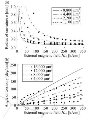
Figure 7: Experimental results. (a) Relationship between external magnetic field and radius of curvature  $\rho$ . (b) Relationship between external magnetic field and angle of torsion  $\eta$ .
