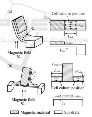
Figure 1: Schematic image of designed microstructure. (a) Microstructure to apply bending deformation. (b) Microstructure to apply torsion deformation.
