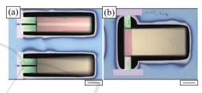
Figure 5: Images of fabricated microstructures. (a) The microstructure to apply bending stimulus. (b) The microstructure to apply torsion stimulus. Scar bars, (a) and (b):  $100 \mu m$ .
