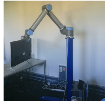
(b) Image of the UR10 in use for the experimental demonstration.
