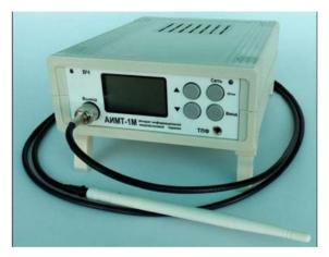
Figure 1: Device for simulating solar microwave radiation in the frequency range (4.0-4.3) GHz.
