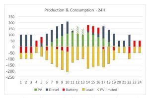
Figure 6: Use Case: Production and Consumption on a day.
