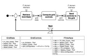
Figure 3: Use case: IT process model in fUML.
