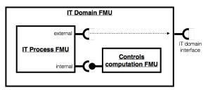
Figure 4: Use case: IT domain FMU composed of the IT process FMU and one out-sided function FMU.
