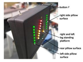
Figure 5: LED display mounted in front of the patient with LED bars and button "P" indicated.
