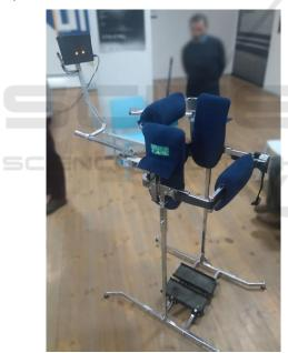
Figure 3: A photograph of the JStep platform with LED display mounted in front of the modified stander.
