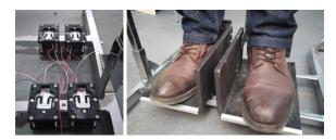
Figure 2: Four YZC-161 load cells bundled to measure weight of the patient (left); standing platforms mounted on the top of the load cells (right).
