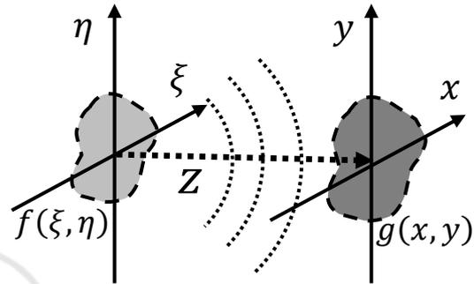
Figure 1: Sketch of a general optical system and its coordinate system.
