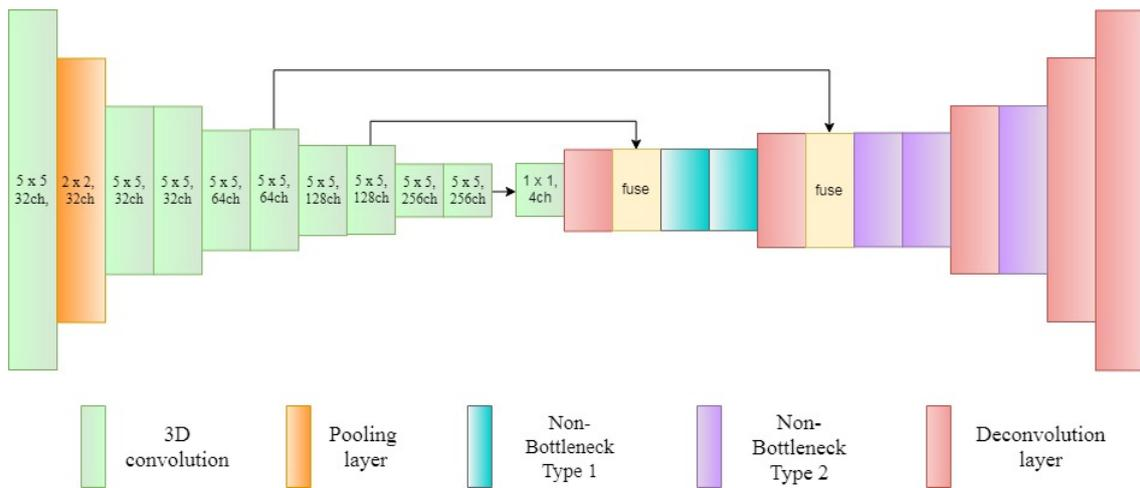
Figure 3: CNN based encoder-decoder architecture used for semantic segmentation task.
