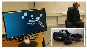
Figure 2: The Ball-throwing level, using the Leap Motion sensor. Inset in the lower-right corner shows the HTC Vive, its controller and the Leap Motion sensor attached to the front of the headset.
