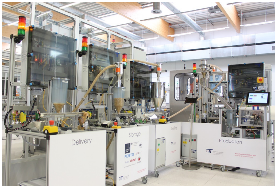
Figure 3: Graphical image of the Versatile Production System of the SmartFactoryOWL. The VPS consists of four different modules (Delivery, Storage, Dosing and Production).
