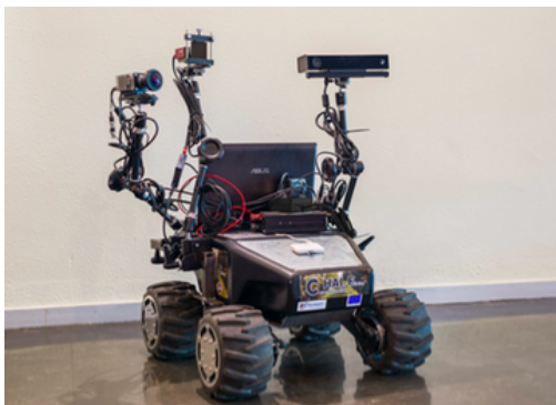
Figure 4: Mobile robot platform used for the acquisition of the POLABOT dataset. It is equipped with the IDS Ucam, PolarCam, Kinect 2 and a NIR camera.
