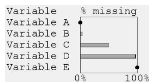
Figure 1: Bars and dots visualization of a scalar. The values for variables A and E are drawn as dots because they are the minimum and maximum of the range (0% and 100% missing, respectively). The bars for variables B and D are drawn using perceptual discontinuity, because the values are very small (0.01%) and large (99.99%), respectively.
