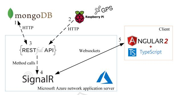
Figure 6: Architecture of the developed system for GPS data visualisation.
