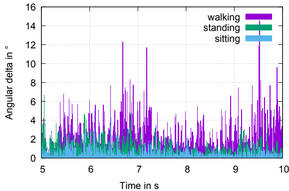
Figure 8: Impact of user behavior on accelerometer readings.
