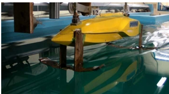
Figure 10: Towing tank test at 12knots speed.
