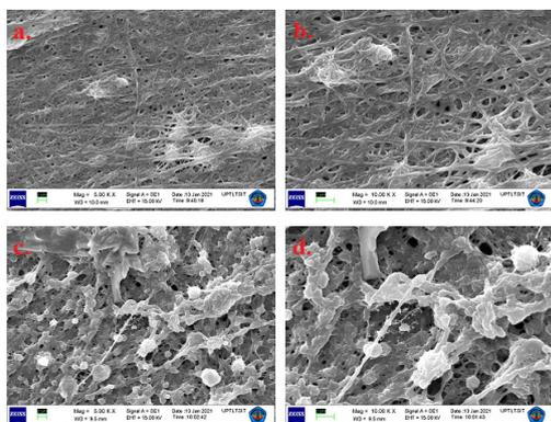
Figure 3. Surface morphology of PEO nanofiber with magnification of (a) 5 Kx, (b) 10 Kx, and PEO/Lignin nanofiber with magnification of (a) 5 Kx, (b) 10 Kx.
