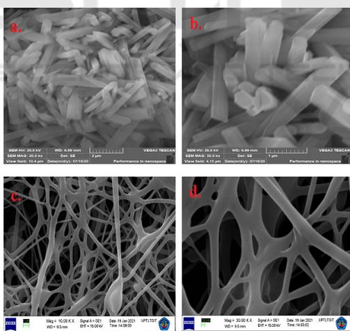
Figure 1. PEO/lignin fiber of various weight ratio surface morphology before emission gas test a) (6: 0) Mag 5 Kx; b) (6: 0) Mag 10 Kx; c) (6: 5) Mag 5 Kx; d) (6: 5) Mag 10 Kx
