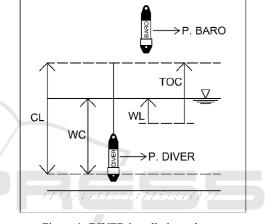
Figure 1: DIVER installation scheme.
