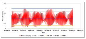
Figure 5: The water level in the parit river  $\rightarrow$  LLWS= 0.
