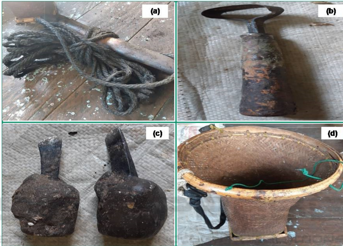
Figure 1. The equipments that are used on tapping of incense sap: (a) Nylon rope stairs, (b) metal chisel, (c) Metal sickle with dull, and (d) bamboo basket.
