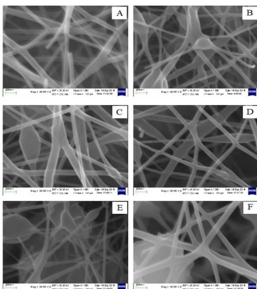
Figure 4: SEM images of PVA 10% (w/v) contained of lignin (a) 0 g (b) 0.5 g, (c) 1.0 g (d) 1.5 g, (e) 2.0 g, (f) 2.5 g.
