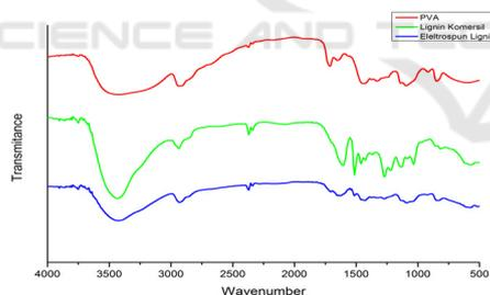
Figure 5: FTIR spectrum of lignin commercial, PVA/lignin, PVA.
