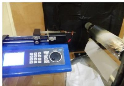
Figure 1: Process of electrospinning PVA/lignin.
