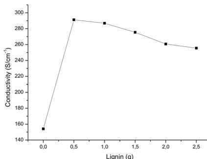
Figure 3: The conductivity of PVA 10% in deionized water/lignin.
