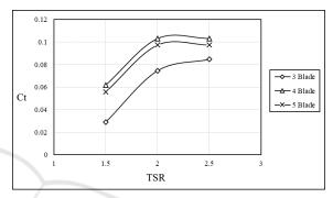
Figure 8: Ct-TSR curve at all the turbine blades.
