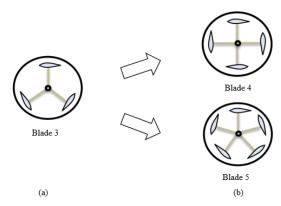
Figure 1: (a) Basic turbine, (b) variations turbine.
