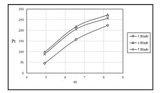
Figure 10: The results of the turbine power.
