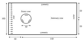
Figure 3: Domain boundary of the turbine model.
