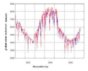
Figure 7: Global horizontal solar radiation estimated from a sunshine duration of the 2003-2005 period, in red the desired outputs, in blue the predicted outputs (simulated).
