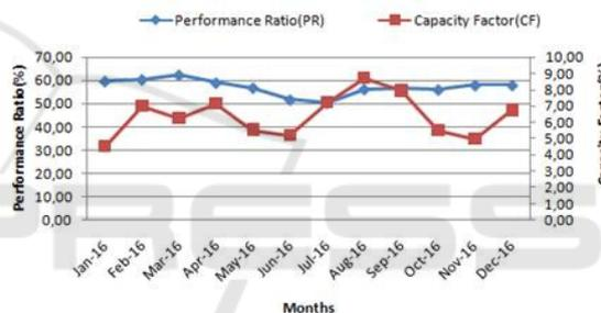
Figure 10: Performance Ratio and Capacity Factor of the a-Si PV system.
