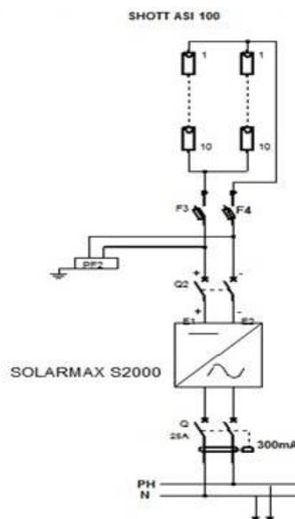
Figure 2: Diagram of the 2.4kWp a-Si grid connected PV plant.
