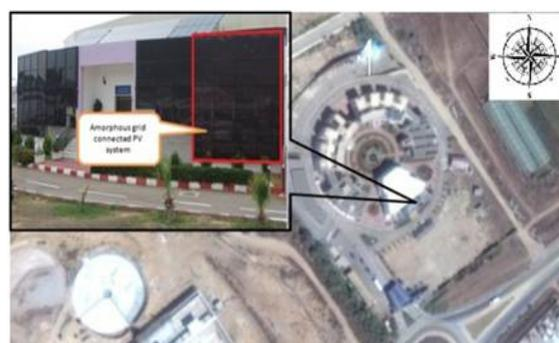
Figure 1: View of the 2.4 kWp amorphous Silicon facade mounted PV plant
