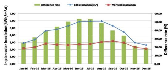
Figure 3: Monthly average daily irradiation respectively on the vertical plan of the PV array and on the optimal angle for the site (36°).
