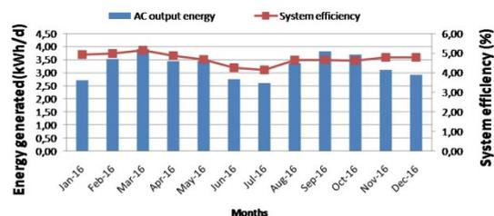
Figure 6: Monthly average AC output energy and efficiency of the a-Si PV system.
