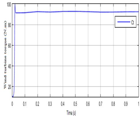
Figure 19: Wind turbine torque with MPPT.
