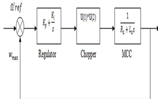
Figure 6: Block diagram of the MCC regulated by a PI.
