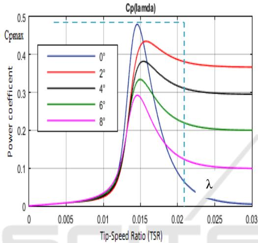
Figure 3: Power coefficient as a function of  $\lambda$ .
