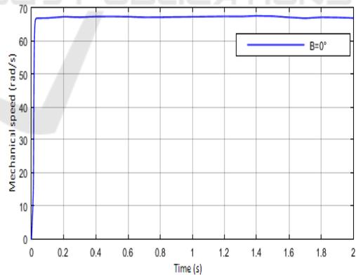
Figure 11: Evolution of the speed of the turbine.
