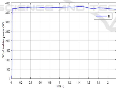
Figure 18: Wind turbine power with MPPT.
