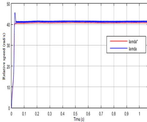
Figure 16: Relative speed with MPPT.
