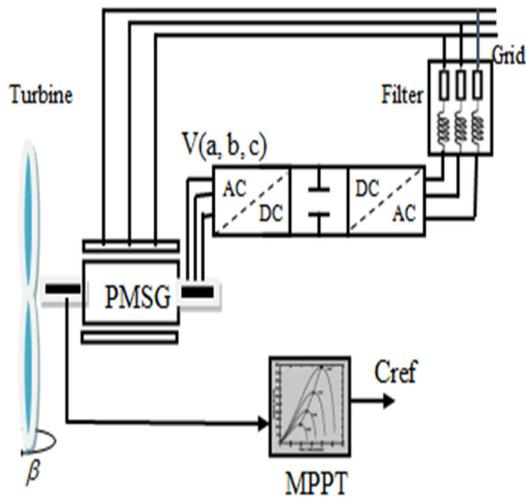
Figure 1: Wind energy conversion system (WECS).
