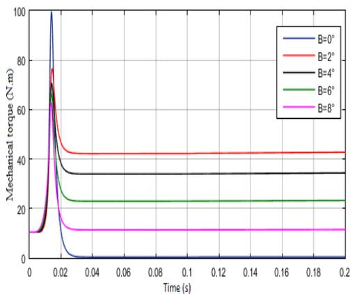
Figure 12: Evolution of turbine torque.
