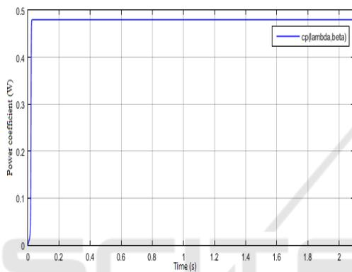
Figure 17: Power coefficient with MPPT.
