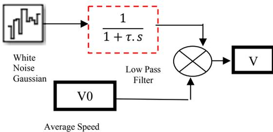
Figure 2: Synoptic diagram of wind reconstruction.
