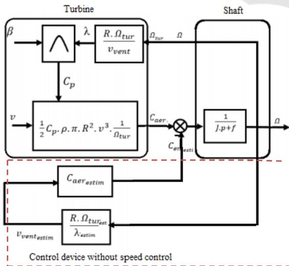
Figure 9: Block diagram of the maximization of the power extracted without servo of speed.
