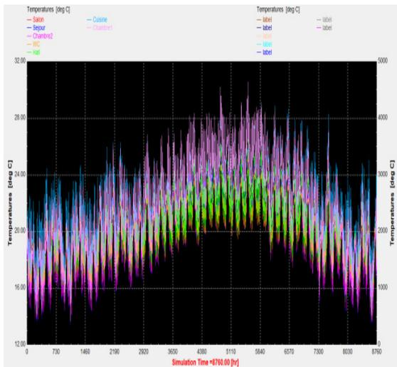
Figure 4: Thermal behavior of the building without heating or cooling system
