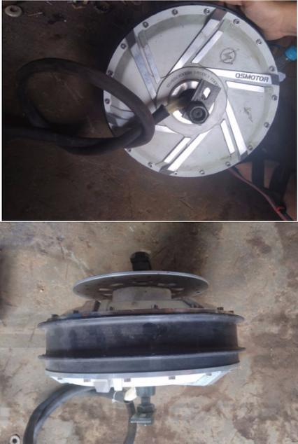
Figure 4: The 3 kW 48 V BLDC motor.
