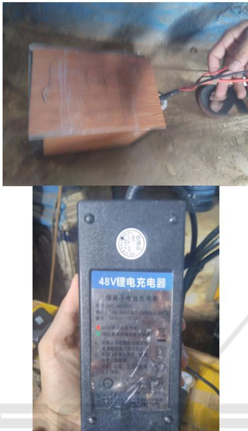
Figure 5: The packed Lithium battery and a charger.
