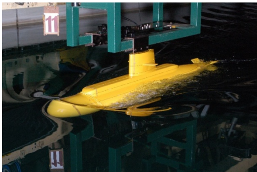
Figure 4: Resistance test at 7 knots surface condition (V = 1.361 m/s).
