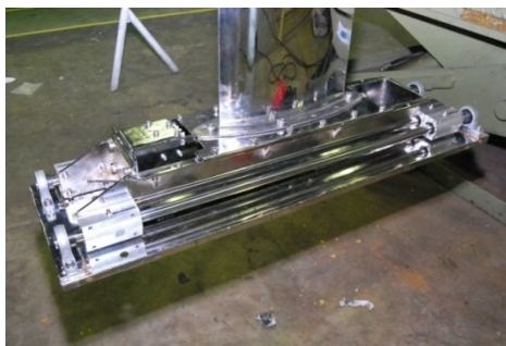
Figure 2: Special dynamometer for measuring resistance force of submarine model.
