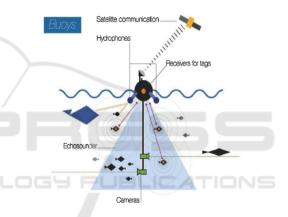
Figure 2: Concept of smart FADs.
