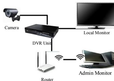
Figure 7: CCTV System Network Topology.
