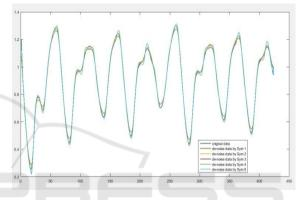
Figure 8: Original data (chaotic Mackey Glass) versus approximated data using denoised wavelet with several orders of Symlets wavelet.
