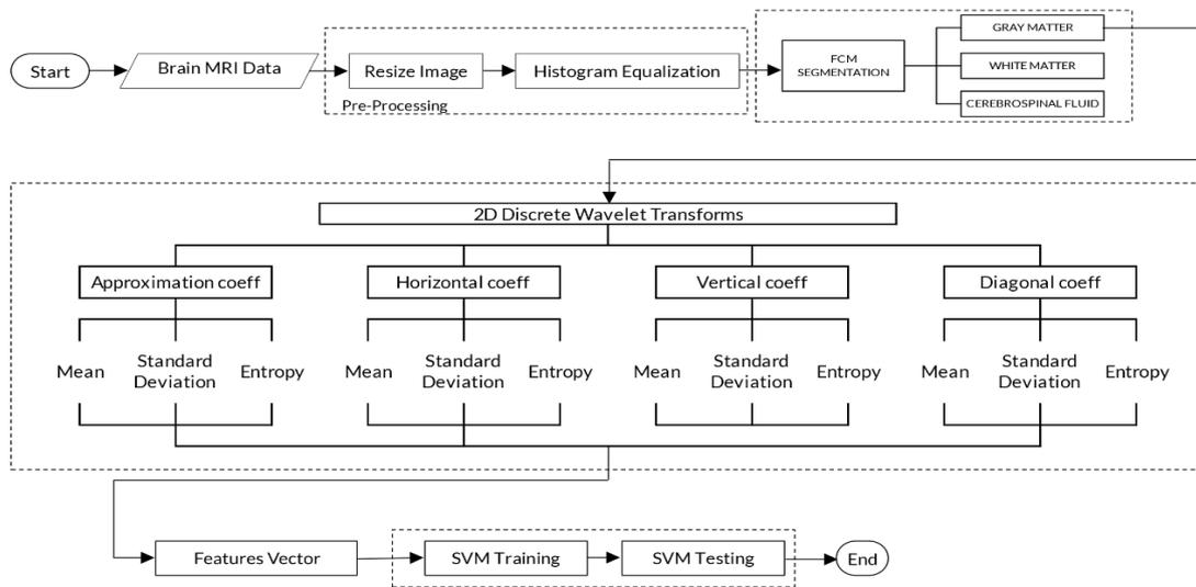
Figure 3: Diagram of the Process
