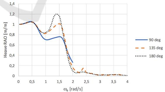
Figure 7: Heave RAOs for 12 knots ship speed with  $90^\circ$ ,  $135^\circ$  and  $180^\circ$  wave headings.
