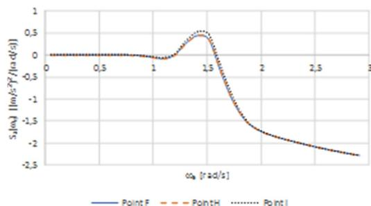
Figure 14: Vertical acceleration spectra at points F (1.0 m fore CG), H (2.0 m fore CG) and I (12.0 m fore CG) for 12 knots ship speed in head waves (truncated at  $\omega_e = 3.0$  rad/s).
