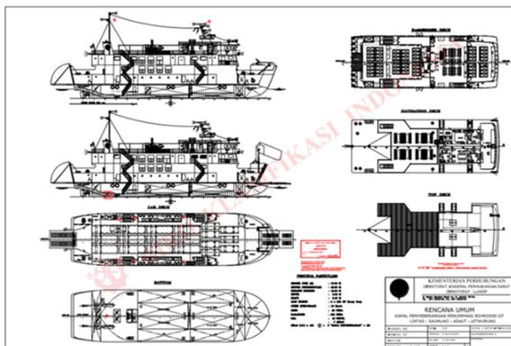
Figure 2: General arrangement of the ro-ro ferry.
