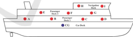
Figure 11: Locations within the ship where the relative motion, the vertical acceleration and the MSI are calculated, denoted by points A, B, ... I.
