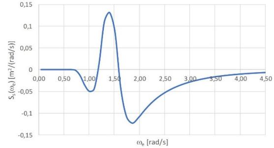
Figure 12: Relative motion spectrum at point I for 12 knots ship speed in head seas.
