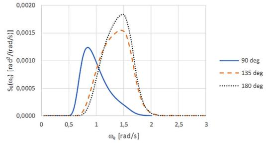
Figure 10: Pitch spectra for 12 knots ship speed with 90°, 135° and 180° wave headings.
