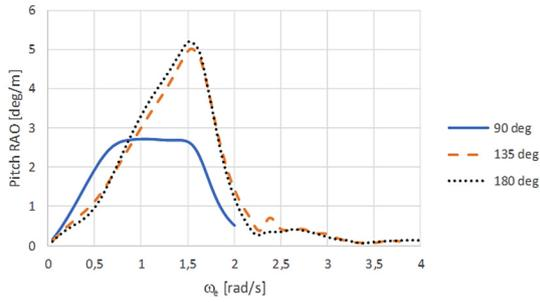
Figure 8: Pitch RAOs for 12 knots ship speed with 90°, 135° and 180° wave headings.
