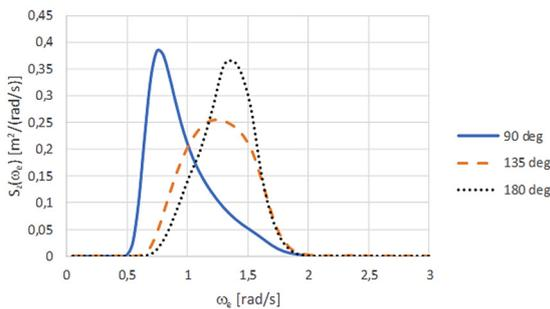
Figure 9: Heave spectra for 12 knots ship speed with 90°, 135° and 180° wave headings.
