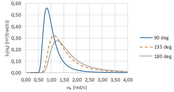
Figure 6: Encounter wave spectra for 12 knots ship speed with  $90^\circ$ ,  $135^\circ$  and  $180^\circ$  wave headings.
