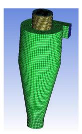
Figure 3: The hexahedral structured grid.
