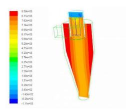
Figure 4: The pressure contour of the internal flow field.
