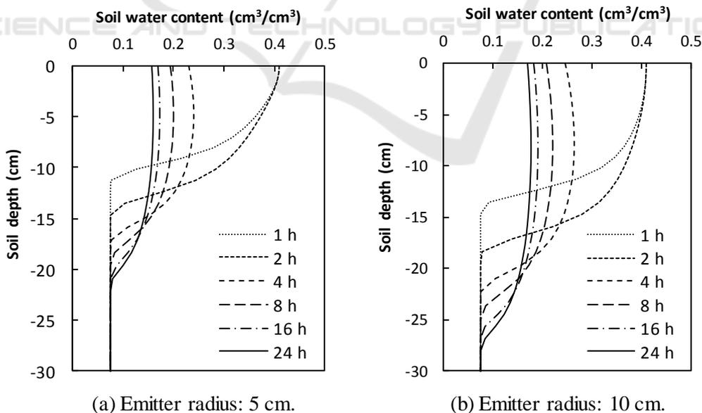
**Figure 2.** The variation of soil water content distribution in the vertical direction with time (irrigation duration: 2 h).
