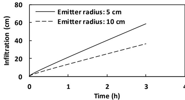
**Figure 1.** The simulated cumulative infiltration under different emitter radii.
