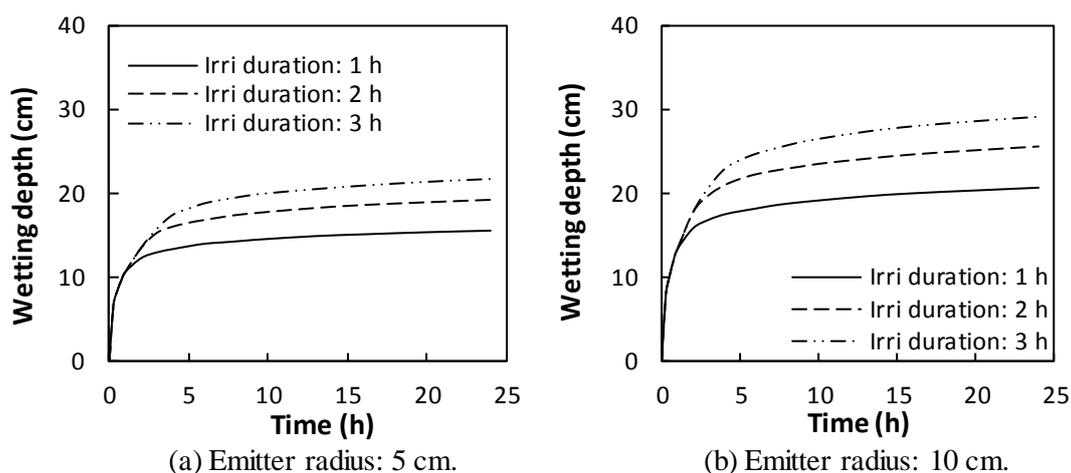
**Figure 4.** Effects of the emitter radius and irrigation duration on the soil wetting depth.
