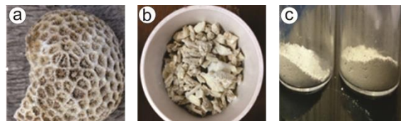
Figure 1: The process of sample preparation (a) coral has been cleaned, (b) coral has been dissolved, (c) coral has been refined.
