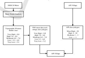
Figure 2: Flow Chart Processing TWI data and API
