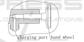
Figure 6: The diagram of electric valve inflatable state.
