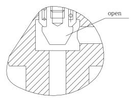
Figure 5: The diagram of electric valve open state.
