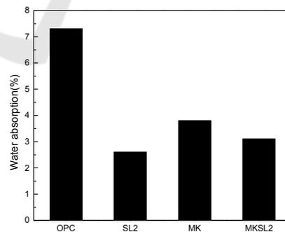
Fig4: Effect of modified metakaolin on water absorption of concrete with water-based organic silicon.
