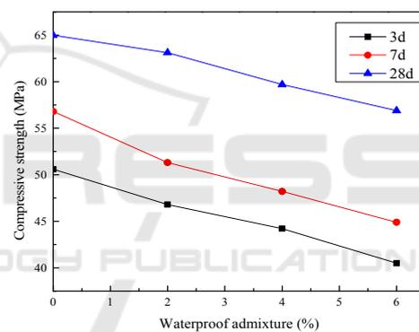
Fig 1: Effect of water-based organic silicon on compressive strength of concrete.
