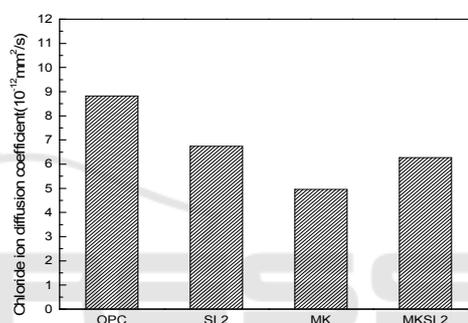
Fig6: Effect of modified metakaolin on chloride diffusion coefficient of concrete with water-based organic silicon.
