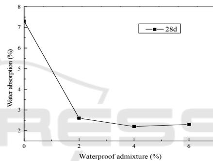
Fig 3:Effect of water-based organic silicon On water absorption of concrete.
