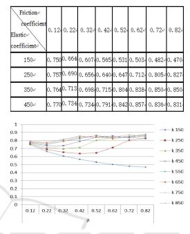
Fig 6The stability time changed with friction coefficient and elasticity coefficient
