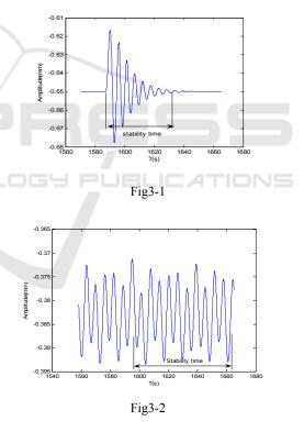
Fig.3Thevibration response at speed of 760 and 800r/min.
