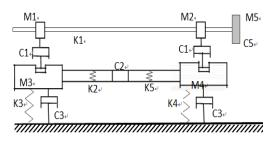
Fig.1 The mechanical model of ship shafting.
