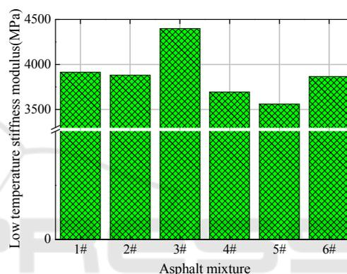
Figure 3 Low temperature stiffness modulus of asphalt mixture
